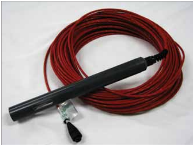
Digital Hydrocarbon Probe
